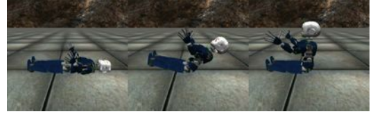
Fig. 7. Screenshots of successful sit-up motion in the SS interaction. The left, middle, and right figures show the initial, intermediate, and final reference of the sit-up, respectively .
